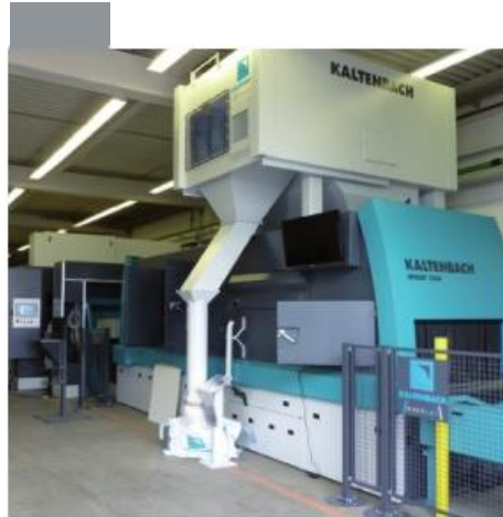
Shot blast and painting unit
